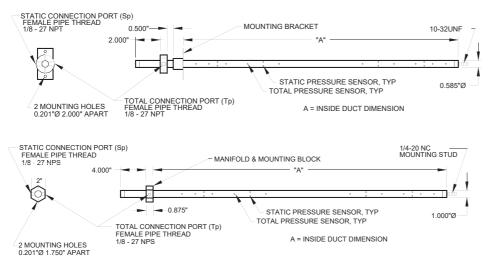
Note: The 0.585 inch diameter probe is used for elements up to 36 inches long and the 1 inch diameter probe is used for elements greater than 36 inches long.
